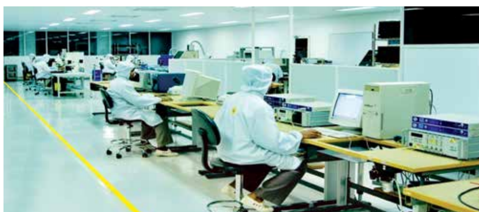
Class 10,000 Clean Room at SFO.
